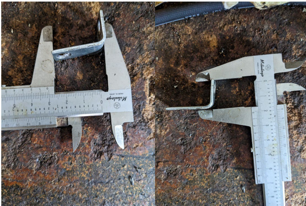
Mounting brackets for T-pieces, mounted on the brake plates
