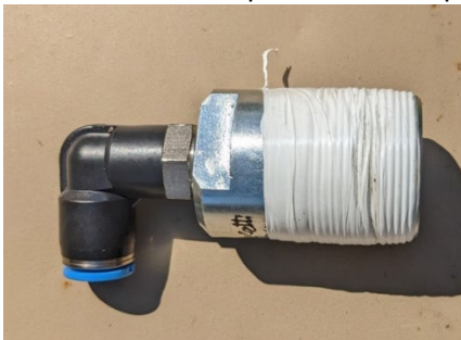
Picture: Buzzetti pole wheel puller M28x1.25, converted to 1/4" hose connection
