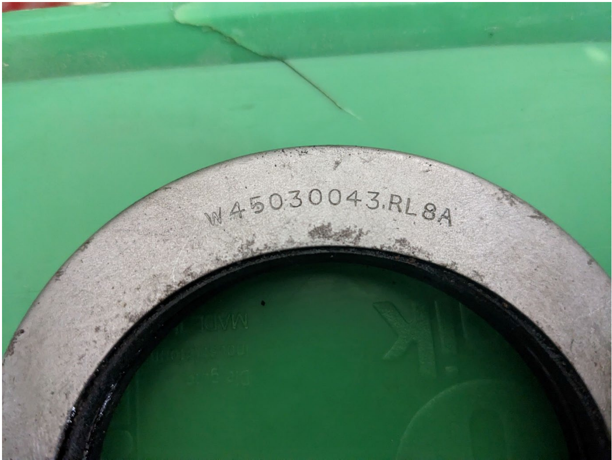
Original shaft seal. Replacement: SKF 30095
